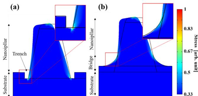
Fig. 2 FEA results of stress distribution in glass nanopillar (a) without bridged structure and (b) with bridged structure.
