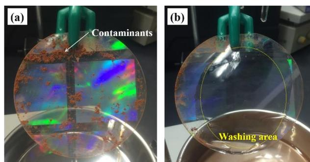
Fig. 5 Self-cleaning demonstration of bridged glass nanopillar. (a) Before washing and (b) after washing.
