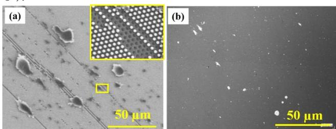
Fig. 4 SEM images of glass nanopillar after friction test. (a) Without bridged structure and (b) with bridged structure. The inset shows magnified image.
