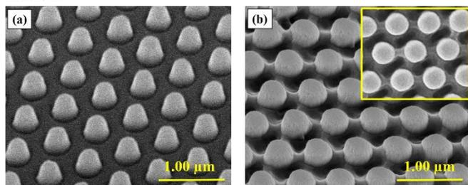
Fig. 3 Tilted view SEM images of glass nanopillar (a) without and (b) with bridged structure. The inset shows top view image.
