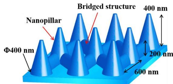
Fig. 1 Design of bridged glass nanopillar.
