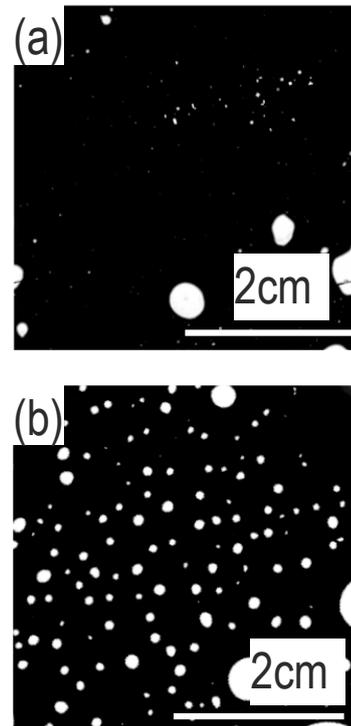
Figure 2: The SAT images of the interfacial voids in the bonding interface by the process 3. The black area is bonded interface and the white spots are the interfacial voids.
