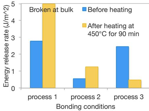
Figure 1: The energy release rate of the bonded interface between the glass and Si substrates by each process. The strength was evaluated by the blade insert test before and after heating at 450 °C for 90 min.
