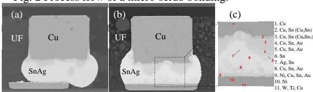
Fig. 3 Cross-sectional SEM image of micro-bump (a) without micro-scrub, (b) with micro-scrub, (c) EDS result.
