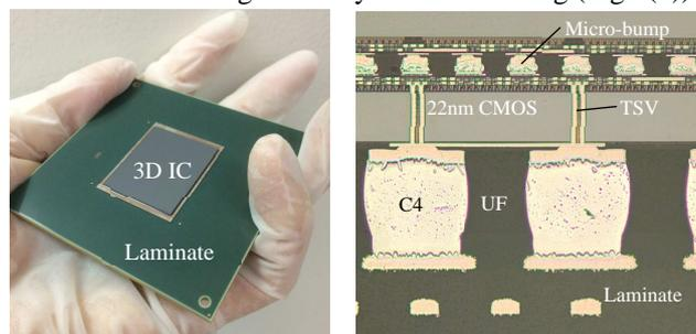
Fig. 4 Large-die 3D IC using 22nm ULK dielectrics (a) after assembly, (b) Cross sectional image.
