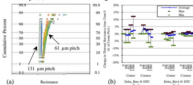
Fig. 5 (a) Resistance measurement over for 3D module, (b) Thermal reliability of TIM1 and die-to-die interfaces.
