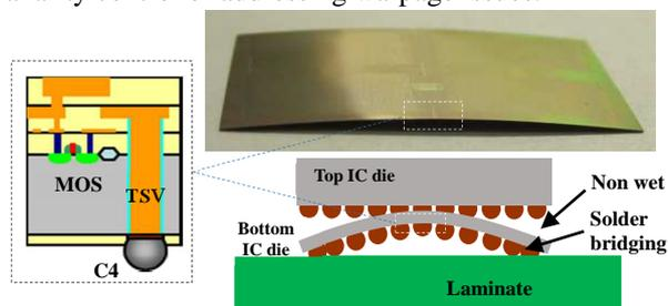
Fig. 1 Warped thin CMOS die causing serious problems to 3D IC packaging.
