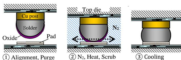
Fig. 2 Process flow of a micro-scrub bonding.
