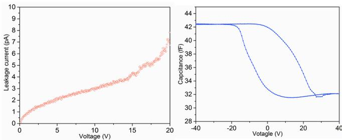
Fig. 2 Electrical measurement results at room temperature. (a) I-V characteristics of a single TSV, (b) C-V characteristics of a MIS trench capacitor.
