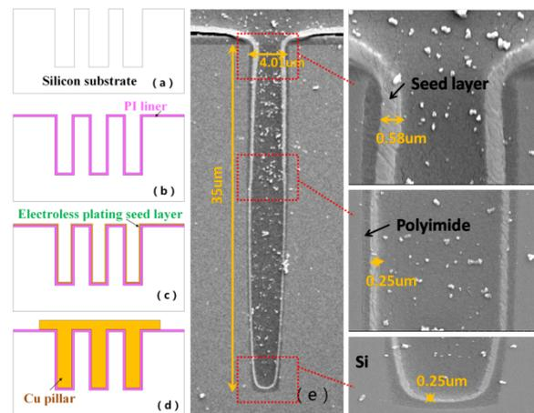
Fig. 1 Schematic TSV fabrication with all-wet processes.
