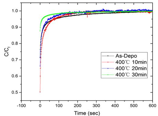
Fig. 3 Measured C-t curves of the trench capacitors after annealing at 400°C and different times.
