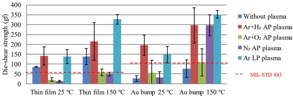
Fig. 2. The results of die-shear test with differences of plasma types, sample shapes and bonding temperature
