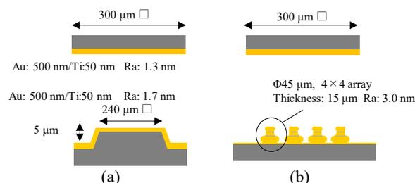
Fig. 1. Schematic diagrams of bonding samples. (a) Au thin film–Au thin film, (b) Au thin film–Au stud bumps.
