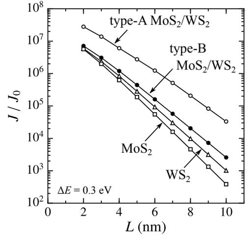
Fig. 5:  $L$  dependence of  $J$  of type-A and type-B  $\text{MoS}_2/\text{WS}_2$  heterojunctions compared with  $\text{MoS}_2$  and  $\text{WS}_2$  homojunctions.
