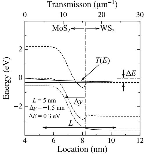
Fig. 2: Band-edge profiles (dashed lines) and transmission function,  $T(E)$ , (solid line) for the type-A  $\text{MoS}_2/\text{WS}_2$  heterojunction. Dotted line shows the applied potential profile (vertically shifted for clarity).
