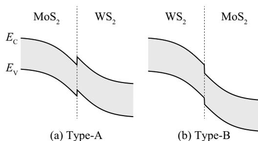
Fig. 1: Two kinds of band profiles for MoS<sub>2</sub>/WS<sub>2</sub> in-plane heterojunctions. (a) Type-A band profile has a potential notch at the heterointerface, while (b) type-B has no potential notch.
