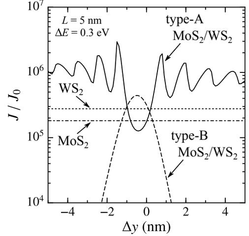
Fig. 4:  $\Delta y$  dependence of  $J$  of type-A and type-B  $\text{MoS}_2/\text{WS}_2$  heterojunctions compared with  $\text{MoS}_2$  and  $\text{WS}_2$  homojunctions.
