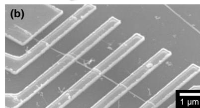
**Fig. 2:** (a) Device schematic and (b) SEM image of a typical 4-terminal device.
