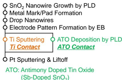
**Fig. 1:** Key fabrication processes of SnO<sub>2</sub> nanowire devices.
