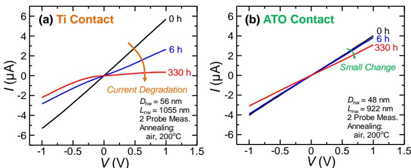
**Fig. 3:** *I-V* characteristics of (a) Ti and (b) heavily Sb-doped SnO<sub>2</sub> (ATO) contact SnO<sub>2</sub> nanowires as fabricated (0 h), after 6- and 330- hours 200°C air annealing. Although the current of Ti contact devices greatly decrease after annealing, that of ATO contact devices only slightly changes due to the increase in resistivity of SnO<sub>2</sub> nanowire channel, indicating stable operations of ATO contact devices at a high temperature.
