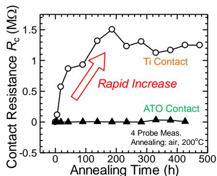
**Fig. 4:** Relationship between contact resistance ( $R_c$ ) and annealing time for Ti and ATO contact devices extracted by 4-probe measurements. The rapid increase in  $R_c$  of Ti contact was clearly observed.
