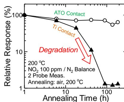
**Fig. 6:** Relationship between relative sensor response to 100 ppm NO<sub>2</sub> and annealing time for Ti and ATO contact SnO<sub>2</sub> nanowire gas sensors. Although the response of Ti contact sensor significantly degrades within 100 hours, that of ATO contact sensor show only small decrease due to oxygen adsorption on SnO<sub>2</sub> nanowire surface.
