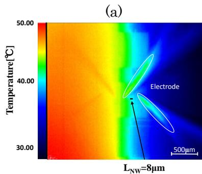
Fig.6 (a) Temperature distribution of the  $\mu$ TEG including a thermography (b) Temperature difference  $\Delta T$  across the SiNW leg
