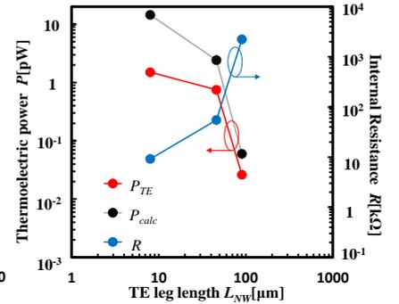
Fig.5  $P_{TE}$ ,  $P_{calc}$ , and  $R \cdot L_{NW}$  characteristics of the p-type  $\mu$ TEG
