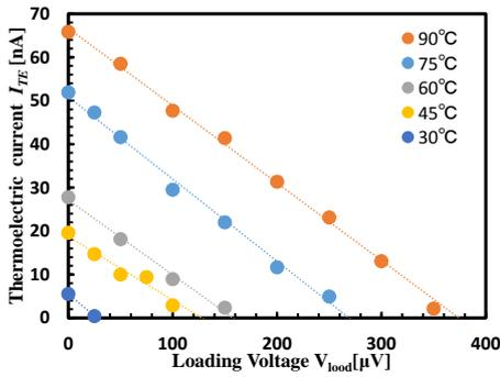
Fig.3  $I_{TE}$   $V_{load}$  characteristics in p-type Si-NW with varying  $T_{hot}$
