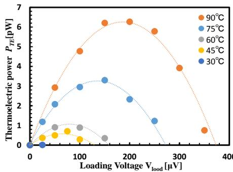
Fig.4  $P_{TE}$   $V_{load}$  characteristics in p-type Si-NW with varying  $T_{hot}$
