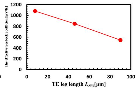
Fig.7 The effective Seebeck coefficient  $-L_{NW}$  characteristics
