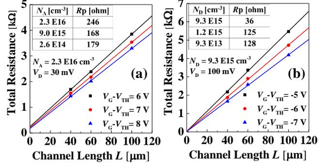
Fig. 4 Relationship between  $R_{\text{total}}$  and  $L$  for (a) n-MOSFETs (b) p-MOSFETs.  $R_{\text{PRS}}$  for all samples are also listed in the tables in each figure.
