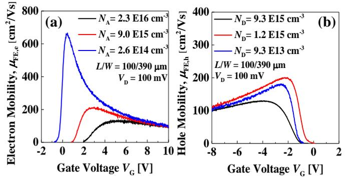
Fig. 5  $\mu_{\text{FE}}-V_{\text{G}}$  plots for (a) n-MOSFETs (b) p-MOSFETs.
