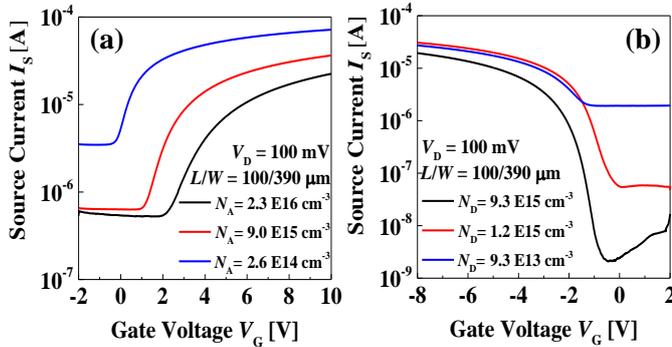
Fig. 3  $I_{\text{S}}-V_{\text{G}}$  characteristics for (a) n-MOSFETs (b) p-MOSFETs.
