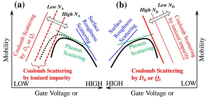
Fig. 6 Schematic model of mobility degradation mechanism for (a) n-MOSFET and (b) p-MOSFET.
