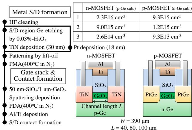
Fig. 1 Fabrication procedures for n- and p-MOSFETs with metal S/D structure.
