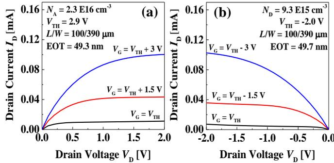
Fig. 2  $I_{\text{D}}-V_{\text{D}}$  characteristics for typical (a) n-MOSFET (b) p-MOSFET.
