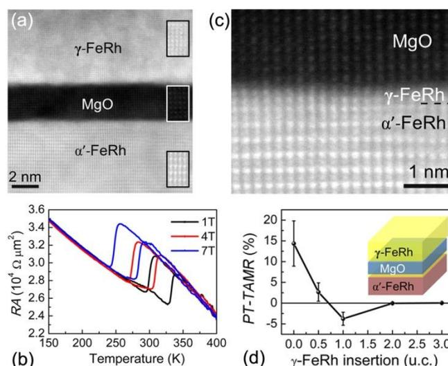
Fig. 1. (a) Cross-sectional z-contrast STEM image of the stack films. (b) Resistance-area (RA) product of the  $\alpha'$ -FeRh/MgO/ $\gamma$ -FeRh junctions as a function of temperature. (c) high resolution STEM Z-contrast image with one unit cell-thick  $\gamma$ -FeRh naturally superimposed at the  $\alpha'$ -FeRh/MgO interface. (d) A summary of the PT-TAMR ratio as a function of the thickness of  $\gamma$ -FeRh insertion.
