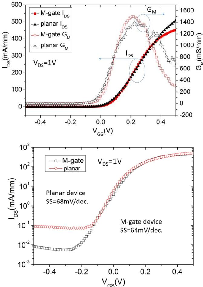
Figure 2. ID/Gm-VG characteristics of  $\pi$ -gate and planar device
