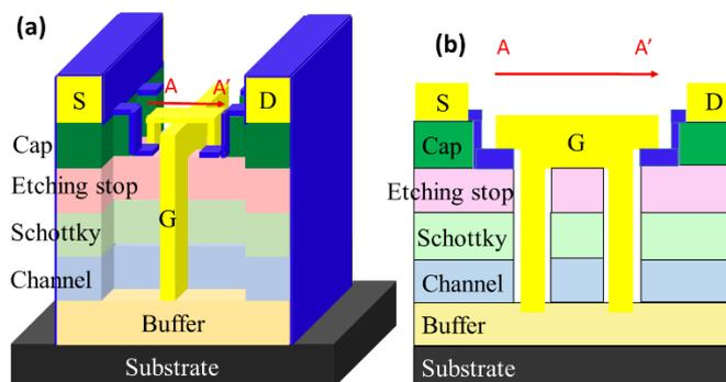
Figure 1. (a) Structure of the device in this study (b) A to A' cross section of the device
