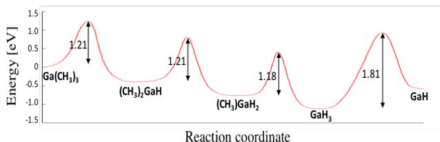
Fig. 1. Activation energy of the main reaction path of TMG at absolute zero.
