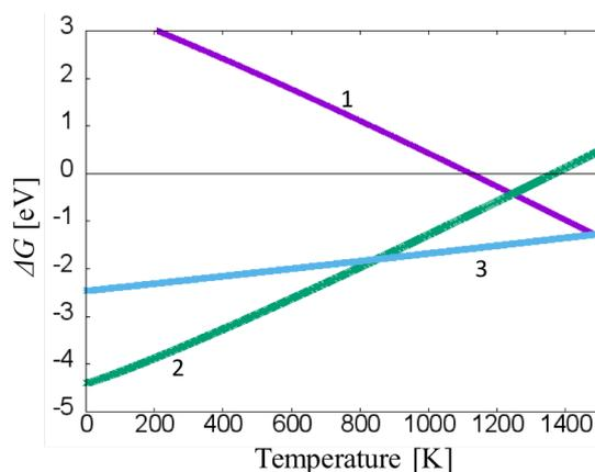
Fig. 3. Calculated formation energy for the three reactions shown in Table I. The purple, green and blue lines are for reactions 1, 2 and 3, respectively.
