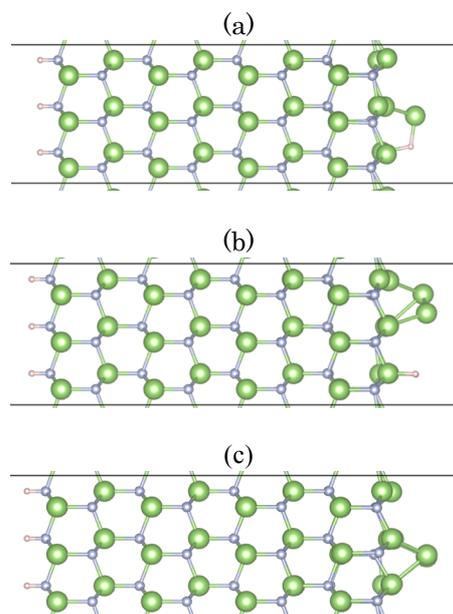
Fig. 2. Slab models where molecules are adsorbed on the (0001) surface. (a), (b) and (c) are the models where one GaH molecule, two GaH molecules and two Ga atoms are adsorbed on the surface, respectively. The green, blue and orange circles show Ga, N and H atoms, respectively.
