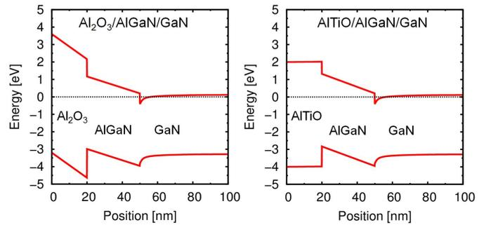
Fig. 5: The band diagrams of the MIS devices, obtained by Poisson-Schrödinger calculation.
