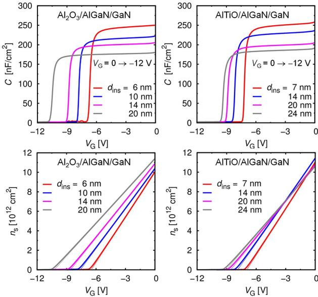
Fig. 2: The capacitance  $C$  and the sheet electron concentration  $n_s$  as functions of the gate voltage  $V_G$ . The measurements were carried out at 1 MHz and under a voltage sweep  $V_G = 0 \rightarrow -12$  V.
