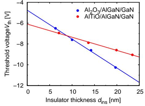
Fig. 3: The threshold voltage  $V_{th}$  as functions of the insulator thickness  $d_{ins}$ .
