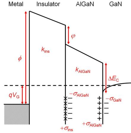
Fig. 4: The schematic band diagram of the MIS devices.
