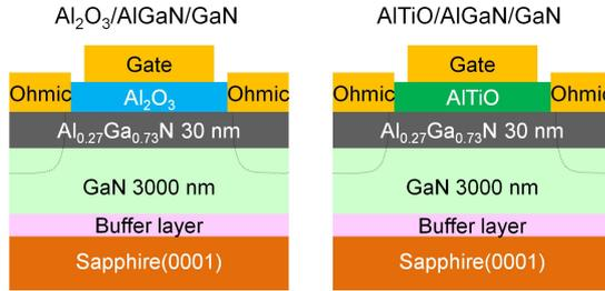
Fig. 1: The schematic cross sections of  $\text{Al}_2\text{O}_3/\text{AlGaIn}/\text{GaN}$  and  $\text{AlTiO}/\text{AlGaIn}/\text{GaN}$  MIS devices.
