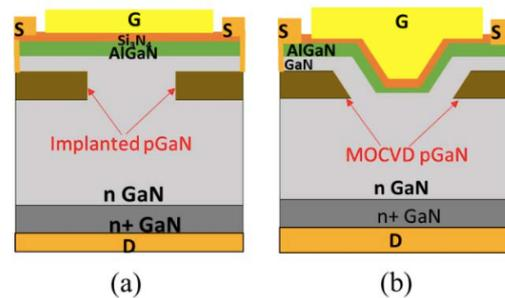
Figure 1. (a) CAVET with implanted [Mg]-GaN as CBLs. (b) Trench CAVET with MOCVD p-GaN as CBLs.
