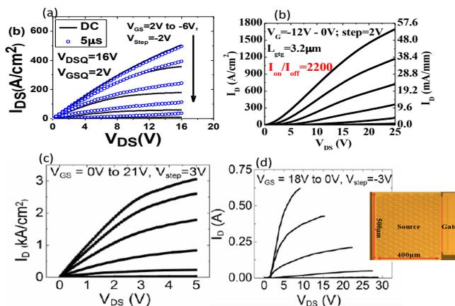
Figure 3. Drain Characteristics of (a) CAVET overlaid with its pulsed I-V characteristics (b) SIT showing triode-like behavior (c) OG-FET unit device and (d) scaled OG-FET
