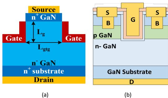
Figure 2. Schematic of (a) SIT without any need for p-type GaN (b) OG-FET with in situ oxide and regrown GaN interlayer
