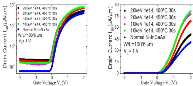
Fig. 4 Transfer characteristics of Ni-InGaAs MOSFETs fabricated with PSD technique in (a) logarithm and (b) linear scale.
