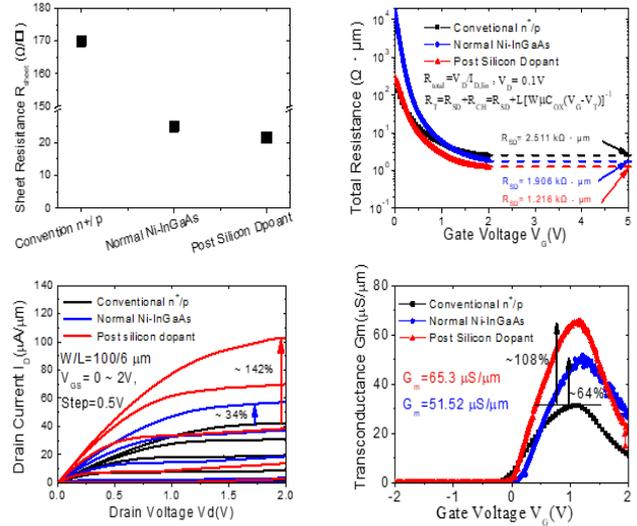
Fig. 5 (a) The sheet resistance and (b) the total resistance in the linear regime ( $V_D = 0.1$  V) as a function of gate voltage for InGaAs MOSFET with or without PSD process. (c) Output and (d) transfer characteristics of InGaAs MOSFETs fabricated with and without PSD process.
