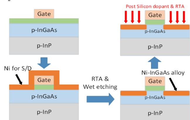
Fig. 1 Schematic diagram of device structure and process flow for the Ni-In<sub>0.53</sub>Ga<sub>0.47</sub>As MOSFET fabrication with PSD technique.
