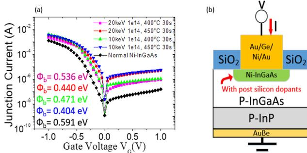
Fig. 2 (a)  $I$ - $V$  electrical characteristics of Ni-In<sub>0.53</sub>Ga<sub>0.47</sub>As/p-In<sub>0.53</sub>Ga<sub>0.47</sub>As diodes fabricated with PDS process. (b) The schematic diagram of the junction cross section.
