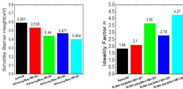
Fig. 3 (a) Electron Schottky barrier height and (b) ideality factor for diodes structures fabricated with a variety of PDS condition.
