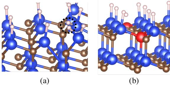
Fig. 3. (a) The H termination model and (b) the N termination model of C vacancies at the 4H-SiC(0001) interface. The large blue, small brown, large red and small white spheres represent the Si, C, N and H atoms, respectively. The circled H atoms are those adsorbed H atoms by annealing.
