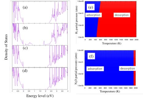
Fig. 4. The density of states of (a) 4H-SiC(0001) interface model, (b) C vacancy model, (c) H terminated model and (d) N termination model. The valence band maximum is set to 0.0eV. (e) H atom adsorption condition and (f) N atom adsorption condition for C vacancy at 4H-SiC(0001) interface.
