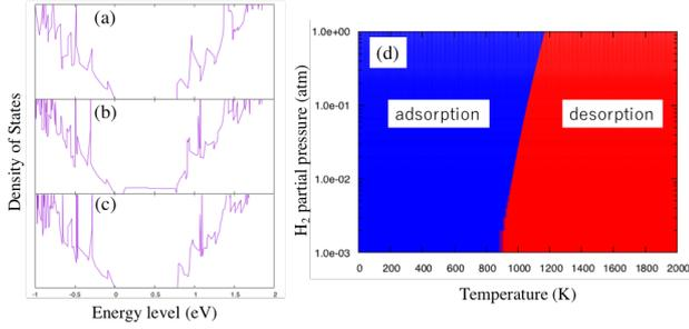
Fig. 2. The density of states of (a) Si(111) interface model, (b) Si vacancy model and (c) H terminated model. The valence band maximum is set to 0.0eV. (d) H atom adsorption conditions for Si vacancies at the Si(111) interface.
