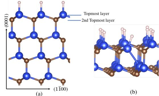
Fig. 1. The calculation model of 4H-SiC (0001) interface. (a) A side view of the 4H-SiC model and (b) the C vacancy model. The large blue, small brown and small white spheres represent the Si atoms, C atoms and H atoms, respectively.
