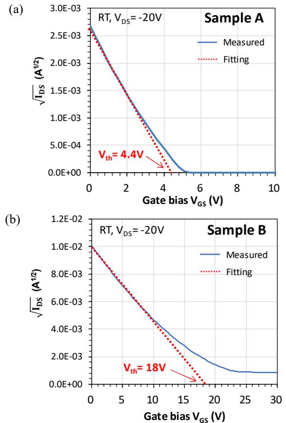
**Figure 3**  $\sqrt{I_{DS}}$ - $V_{GS}$  characteristics of (a) sample A and (b) sample B.
