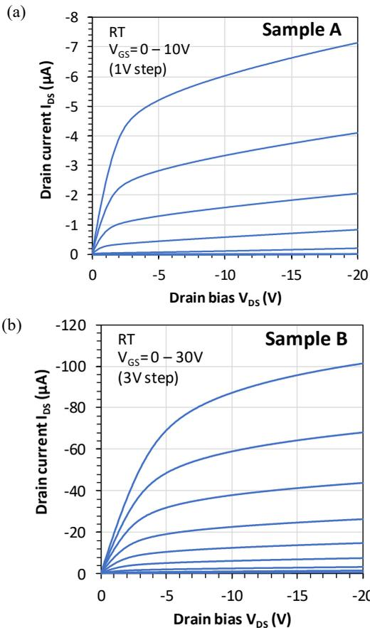
**Figure 2**  $I_{DS}$ - $V_{DS}$  characteristics of (a) sample A and (b) sample B.
