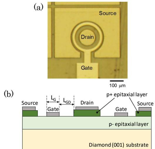
**Figure 1** (a) Top view and (b) cross sectional figure of the diamond MESFET structure.
