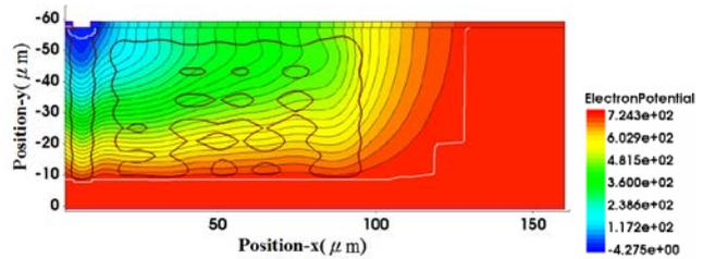
Fig. 6 Potential contours in a double implant structure with both lateral and vertical grading.
