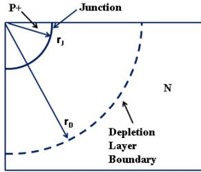
Fig. 1. Structure of a cylindrical PN junction.
