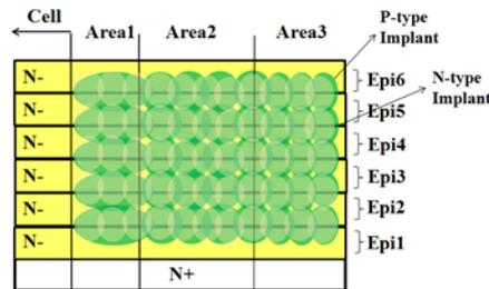
Fig. 3 Doping distribution after thermal diffusion with both P-type and N-type implants introduced in the termination
