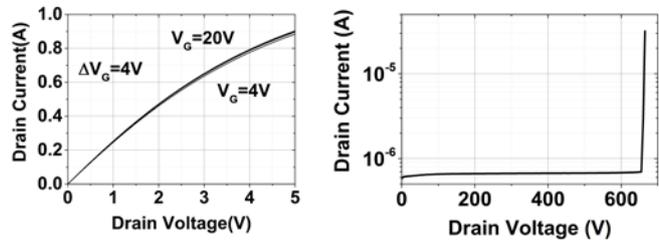
Fig. 7 The measured (a)  $I_D$ - $V_D$  (b)  $BV$  of a fabricated device.
