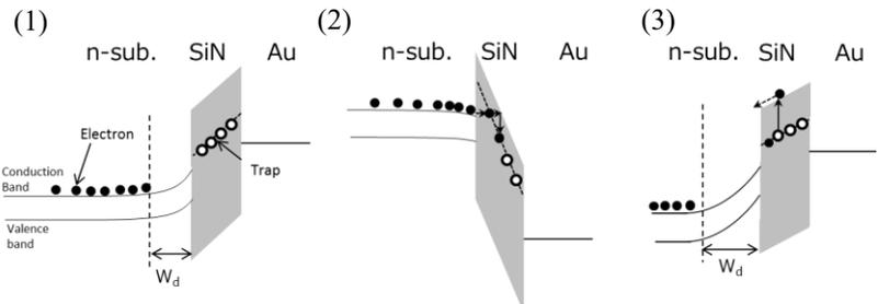
**Fig.5** Energy bands and electron occupancy of SiN film in an MIS capacitor in (1) initial phase with a quiescent bias  $V_r$ , (2) capture phase with a bias  $V_p$  and (3) emission phase with a bias  $V_r$  corresponding to Fig.2.
