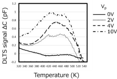
**Fig.6** DLTS spectra measured by applying various injection pulse voltage ( $V_p$ ). The intensity of DLTS signal increases with bias voltage  $V_p$ .
