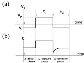
**Fig.2** Illustration of (a) sequence of the bias voltage and (b) the capacitance change during DLTS measurement.
