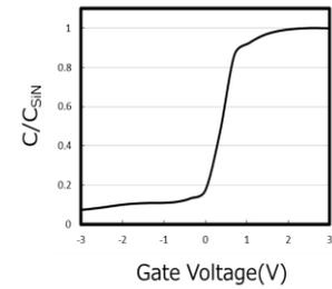
**Fig.3** C-V curve of the MIS capacitor.
