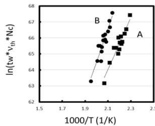
**Fig.7** Arrhenius plots of two traps observed in MIS capacitor for the determination of energy levels and capture cross-sections of the traps.
