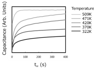
**Fig.4** Temperature dependence of the capacitance transient during emission phase (3) in Fig.2 with  $V_p=2V$ .
