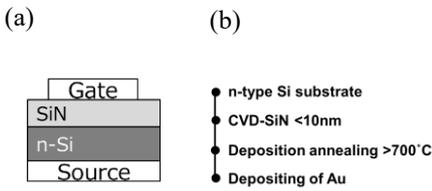
**Fig.1** (a) Structure and (b) process flow of the MIS capacitor for DLTS measurement.
