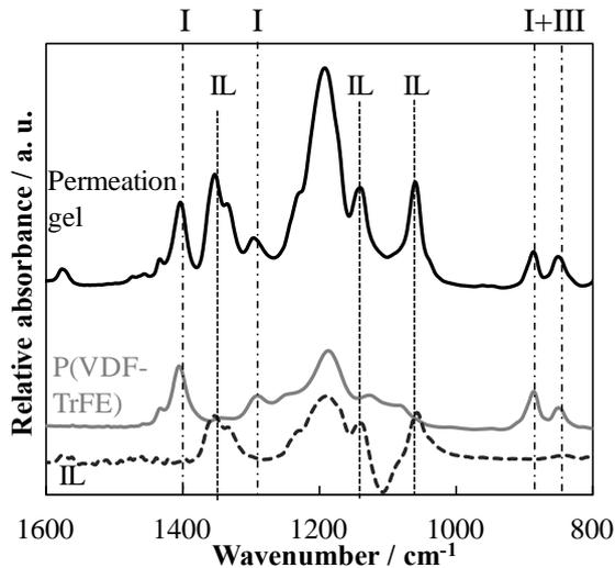
Fig. 2. FT-IR spectra of P(VDF-TrFE)/IL permeation gel, P(VDF-TrFE) thin film and IL.
