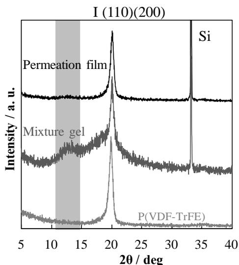
Fig. 1. XRD patterns of P(VDF-TrFE)/IL permeation gel, mixture gel, and P(VDF-TrFE) thin film.
