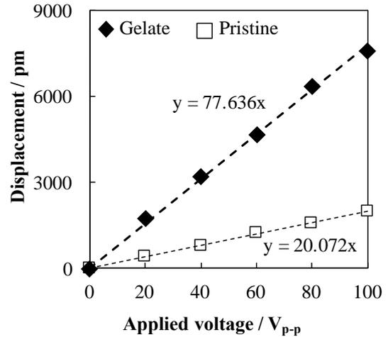
Fig. 4. Piezoelectric displacements of the P(VDF-TrFE) thin films before and after gelation.
