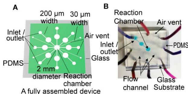
Fig. 1 Microfluidic device for solution exchange. (A) Top view. (B) Photograph of the device with silicone tubes.
