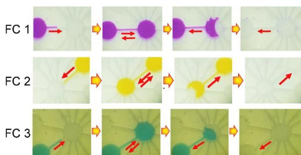
Fig. 2. Images that show sequential exchange of solutions in the microfluidic device. F.C.: Flow Channel.
