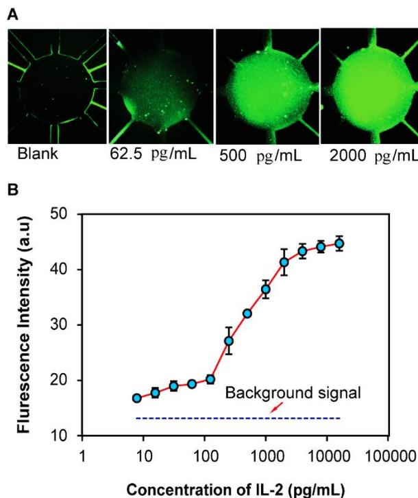
Fig. 3 (A) Optical microscope images of fluorescence from the reaction chamber observed with IL-2 of different concentrations. (B) Dependence of fluorescence intensity on IL-2 concentration. Error bars represent means  $\pm$  standard deviation for 3 replicates.
