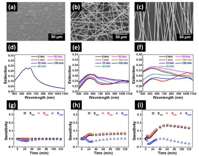
**Fig. 1 (a-c)** The microstructures of various sensing chips, including (a) Type I: P3HT/PMMA film, (b) Type II: random P3HT/PMMA fiber and (c) Type III: aligned P3HT/PMMA fiber, observed by SEM. **(d-f)** Extinction spectra of various sensing chips, including (d) Type I, (e) Type II, and (f) Type III. **(g-i)** The Sensitivities of various sensing chips, including (g) Type I, (h) Type II, and (i) Type III, exposed to saturated toluene for different time.
