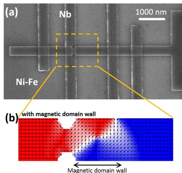
Fig. 2 (a) SEM image of the fabricated sample and (b) result of the micromagnetic simulation of a Ni-Fe wire.
