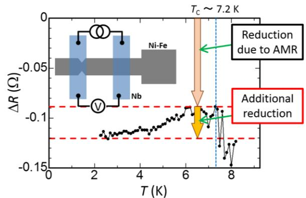
Fig. 4 Temperature dependence of the difference of the Ni-Fe resistance between with and without the magnetic domain wall. The inset shows the probe configuration for the measurement.
