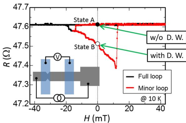
Fig. 3 Magnetic field dependence of resistance of Ni-Fe. The difference of the resistance between state A and state B is due to the anisotropic magneto-resistance. The inset shows the probe configuration for the measurement.
