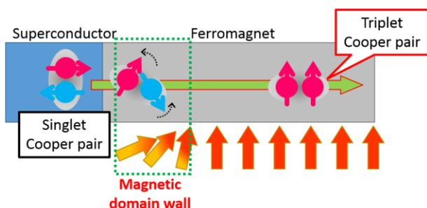
Fig. 1 Conversion of Cooper pair from singlet state to triplet state through magnetic domain wall.
