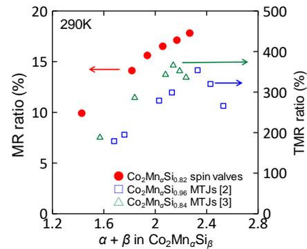
Fig. 3. Comparison of the MR ratios of CMS-based spin valves at 290 K as a function of  $\alpha + \beta$  with the TMR ratios of  $\text{Co}_2\text{Mn}_\alpha\text{Si}_\beta/\text{MgO}/\text{Co}_2\text{Mn}_\alpha\text{Si}_\beta$  MTJs at 290 K as a function of  $\alpha + \beta$ . The MR ratios of the spin valves showed a tendency similar to the MTJs.
