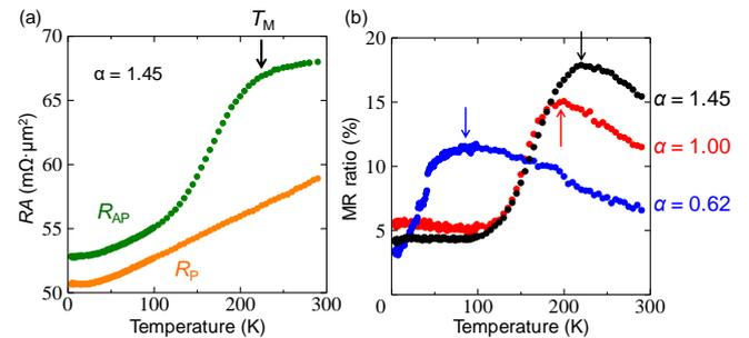
Fig. 2. (a) Temperature dependence of  $R_{AP}$  and  $R_P$  for a CMS/CoFe/Ag/CoFe/CMS spin valve with Mn-rich ( $\alpha = 1.45$ ) CMS electrodes, and (b) temperature dependence of MR ratio for  $\alpha = 0.62, 1.00,$  and  $1.45$ .
