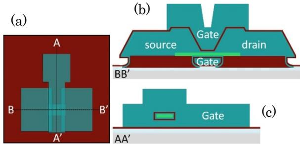
Fig. 1 (a) Top and cross-sectional views along (b) BB' and (c) AA' directions for the Tuber-FET.
