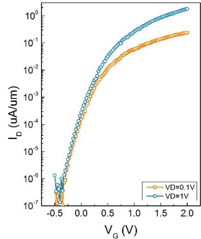
Fig. 5 Transfer characteristics of a Tube-FET.
