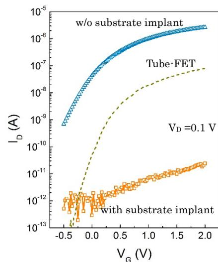
Fig. 6 Transfer characteristics of parasitic transistors with and without substrate implant and the Tube-FET (Fig. 5) measured at  $V_D = 0.1V$ .
