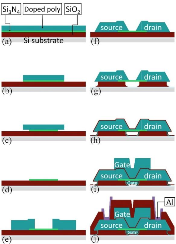
Fig. 2 Process flow of the Tube-FET.
