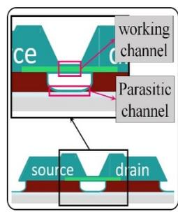
Fig. 3 Existence of a parasitic channel in the Tube-FET.
