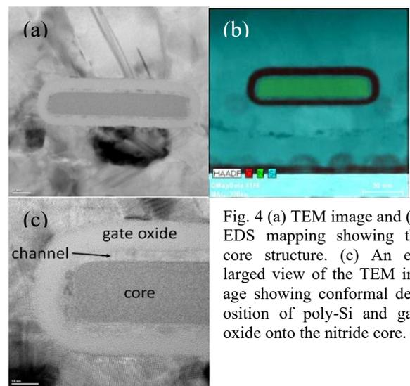
Fig. 4 (a) TEM image and (b) EDS mapping showing the core structure. (c) An enlarged view of the TEM image showing conformal deposition of poly-Si and gate oxide onto the nitride core.
