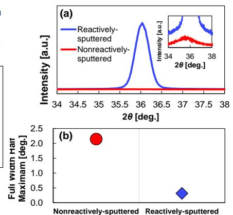
Fig.6 X-ray diffraction (XRD) measurement results. (a) XRD spectra of nonreactively-sputtered AlN film and reactively-sputtered AlN film. (b) Full width half maximum of the AlN (0002)
