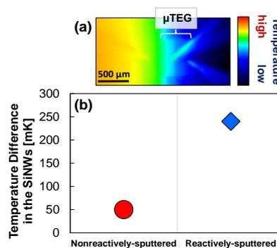
Fig.5 (a) Thermography image of the  $\mu$ TEG (b) Temperature difference between both ends of the SiNWs of the  $\mu$ TEGs with two different types of AlN TC films.
