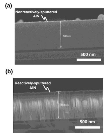
Fig.3 Cross-sectional images of two different types of AlN film. (a) Nonreactively-sputtered AlN (b) Reactively-sputtered AlN
