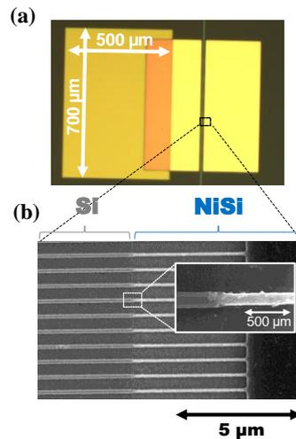
Fig.2 (a) Optical microscopy image of the  $\mu$ TEG. (b) SEM image of the Si nanowire (SiNW) and NiSi pad of the  $\mu$ TEG.
