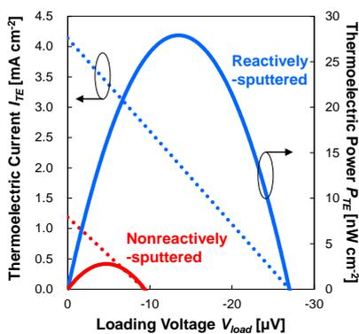
Fig.4  $I_{TE}-V_{load}$  and  $P_{TE}-V_{load}$  characteristic of the  $\mu$ TEG with nonreactively-sputtered AlN TC film (red line) and reactively-sputtered AlN TC film (blue line).
