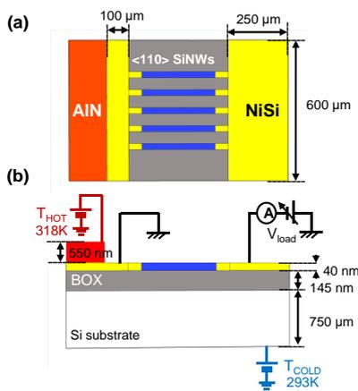
Fig.1 Schematic diagrams of our fabricated Si nanowire-based  $\mu$ TEG. (a) Top-view. (b) Side-view.
