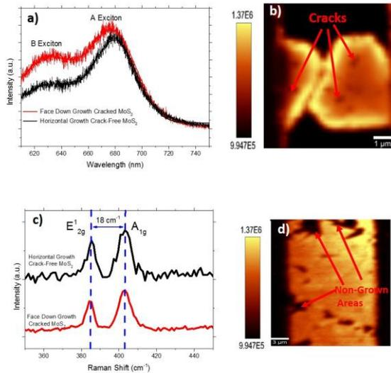
**Fig 2.** a) Single PL spectrum of cracked MoS<sub>2</sub> in the device channel, b) PL map of cracked MoS<sub>2</sub> in the device channel, c) Single Raman spectrums of cracked and crack-free MoS<sub>2</sub> in the device channel and d) PL map of crack-free MoS<sub>2</sub> in the device Channel.
