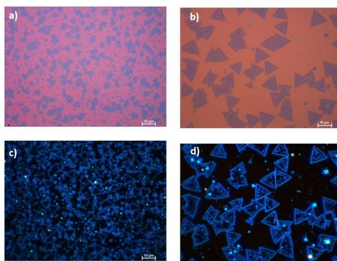
**Fig 1.** Bright and dark-field microscope images of H (a and c) and FD (b and d) grown MoS<sub>2</sub> flakes.
