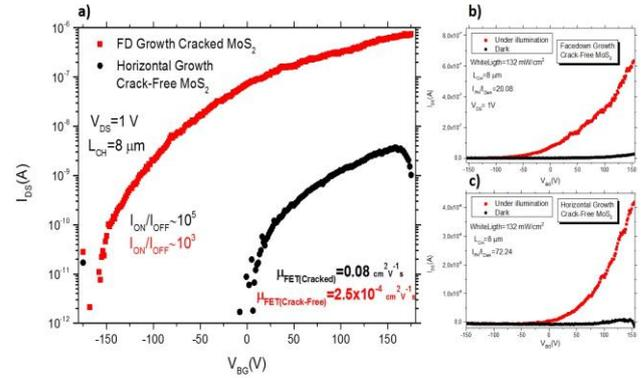
**Fig 3.** Transfer curve (I<sub>DS</sub>-V<sub>BG</sub>) of cracked FD grown and crack-free H grown MoS<sub>2</sub> (a), Gating response of cracked device(b) and crack-free device (c) under dark and illuminated conditions.
