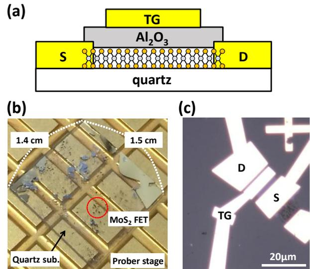
**Fig. 1** (a) schematic of monolayer MoS<sub>2</sub> FET on quartz substrate. (b) Optical image of the quartz substrate. (c) Optical image of magnified MoS<sub>2</sub> device.
