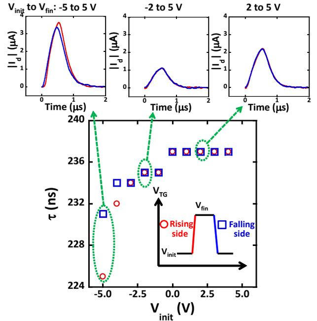
**Fig. 4**  $\tau$  as a function of  $V_{init}$  for rising and falling sides. Top three figures compares absolute value of  $I_d$  as a function of time for both rising and falling sides at different  $V_{init}$ .
