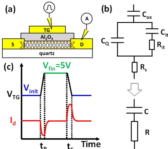
**Fig. 3** (a) Schematic of measurement setup. (b) Equivalent circuit of measured system and simplified circuit. (c) Schematic of applied  $V_{TG}$  and expected  $I_d$  response.
