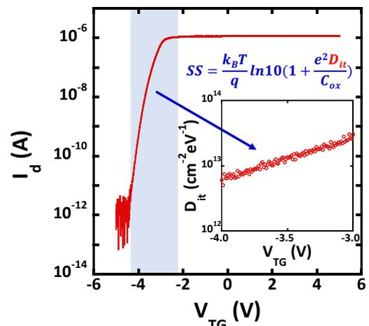
**Fig. 2** DC  $I_d$ - $V_{TG}$  transfer characteristics. (inset)  $D_{it}$  near the conduction band edge as a function of  $V_{TG}$ .
