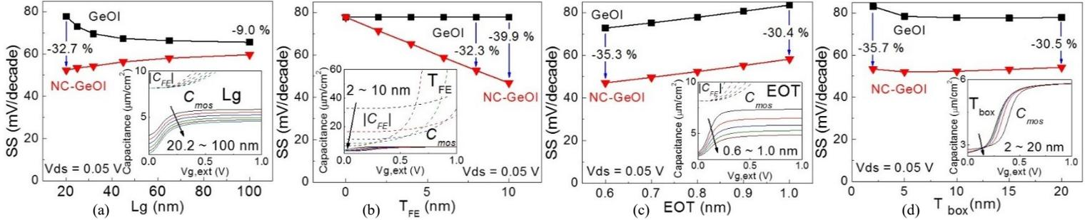
Fig. 4. Impacts of (a)  $L_g$ , (b)  $T_{FE}$ , (c) EOT and (d)  $T_{box}$  on the SS and the capacitances at  $V_{ds} = 0.05$  V.  $C_{mos}$  is the capacitance of the device underneath the ferroelectric layer and  $|C_{FEI}|$  is the capacitance of ferroelectric layer. For NC-GeOI MOSFET at  $V_{g,ext} = 0$  V,  $C_{mos}$  should be close to its  $|C_{FEI}|$  to achieve higher  $A_V$  and larger improvement in SS compared to the baseline GeOI MOSFET.
