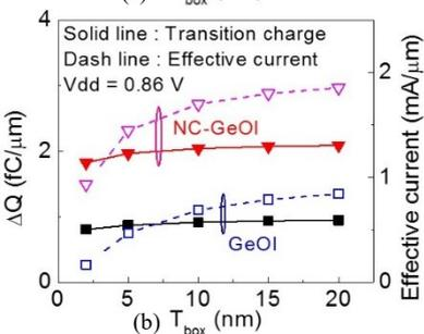
Fig. 7. (a) Impact of  $T_{box}$  on the switching time, (b)  $\Delta Q$  and  $I_{eff}$ . GeOI and NC-GeOI MOSFETs with thinner  $T_{box}$  show larger switching time because of degraded  $I_{eff}$ . Compared to GeOI MOSFET with  $T_{box} = 2$  nm, NC-GeOI MOSFET still exhibits better switching time due to larger  $I_{eff}$ .
