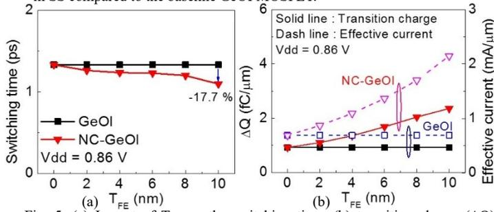
Fig. 5. (a) Impact of  $T_{FE}$  on the switching time, (b) transition charge ( $\Delta Q$ ) and effective current ( $I_{eff}$ ). NC-GeOI MOSFETs with thicker  $T_{FE}$  show lower switching time than GeOI MOSFETs, because NC-GeOI MOSFETs show much larger  $I_{eff}$  in spite of larger  $\Delta Q$  compared with the GeOI MOSFETs.
