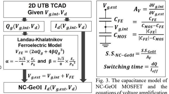
Fig. 2. 2D TCAD GeOI MOSFET simulation coupled with 1D-LK equation is used to model NC-GeOI MOSFET. [5]
