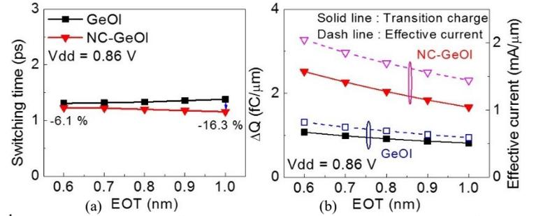
Fig. 6. (a) Impact of EOT on the switching time, (b)  $\Delta Q$  and  $I_{eff}$ . As EOT scales, NC-GeOI MOSFETs show slightly increase in switching time because the increase in  $\Delta Q$  is more than the increase in  $I_{eff}$  as EOT reduces.
