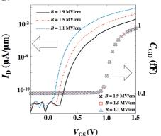
Fig. 5.  $I_{\rm D}$ - $V_{\rm GS}$  and  $C_{\rm GD}$ - $V_{\rm GS}$  curves of n-type TFETs w/ the drain offset for B = 1.1, 1.5 and 1.9 MV/cm.
