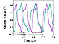
Fig. 3. Output waveforms of the  $3^{rd}$  stage CTFET of ROs w/ and w/o the drain offset.
