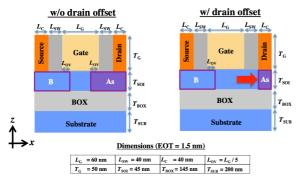
Fig. 1. Schematic figure of the n-type TFET w/ (Left) and w/o (Right) the drain-offset.
