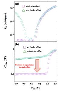
Fig. 2. (a)  $I_{\rm D}$ - $V_{\rm GS}$  curves and (b)  $C_{\rm GD}$ - $V_{\rm GS}$  curves of n-type TFETs w/ and w/o the drain offset.
