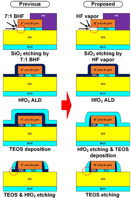
Fig. 2. Key processes modification for fabricating improved HG TFETs.
