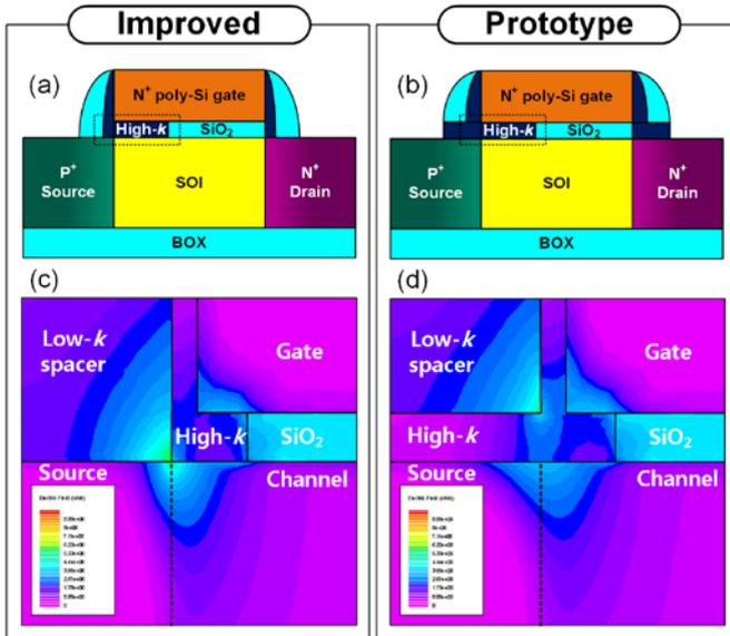
Fig. 1. Comparison of prototype and improved HG TFET. Improved HG TFETs' (a) Device structure. (b) Electric field contour near source-channel junction. And prototype HG TFETs' (c) Device structure. (d) Electric field contour near source-channel junction. The improved HG TFET is more robust to fringing field effect and electric field is concentrated near the junction.
