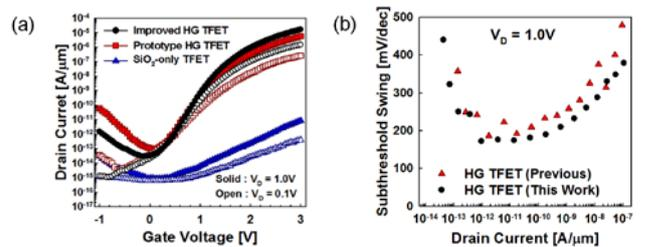
Fig. 4. (a) Transfer characteristics of the improved and prototype HG TFETs and SiO<sub>2</sub>-only TFETs. (b)  $SS$  of the improved and prototype HG TFETs in terms of  $I_D$ .
