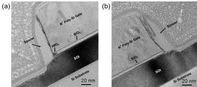
Fig. 3. Cross-sectional TEM image of the fabricated HG TFET in (a) source-side and (b) drain-side.
