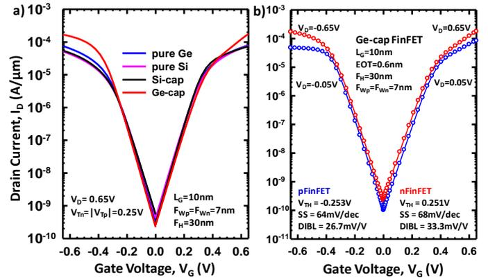
Fig. 2 a) Comparison of  $I_D$ - $V_G$  curve of pure Si, pure Ge, Si-cap, and Ge-cap FinFET and b) transfer characteristics  $I_D$ - $V_G$  curve of Ge-cap QW FinFET with  $L_G=10\text{nm}$ ,  $F_H=30\text{nm}$ , and  $F_{wn}=F_{wp}=7\text{nm}$
