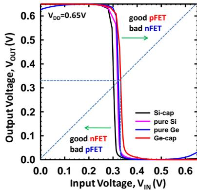
Fig. 5 Comparison of voltage transfer characteristics (VTC) of pure Si, pure Ge, Si-cap, and Ge-cap FinFET CMOS inverter with  $V_{DD}=0.65\text{V}$
