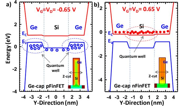
Fig. 4 Band diagram of simulated Ge-cap QW a) pFinFET and b) nFinFET under on-state condition ( $|V_D|=|V_G|=0.65\text{V}$ )
