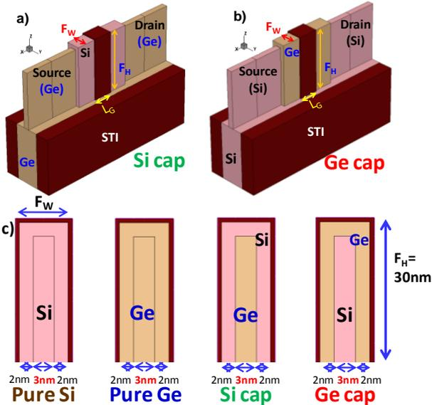
Fig. 1 Device structure of simulated a) Si-cap b) Ge-cap FinFET, and c) cross-section of pure Si, pure Ge, Si-cap, and Ge-cap FinFET
