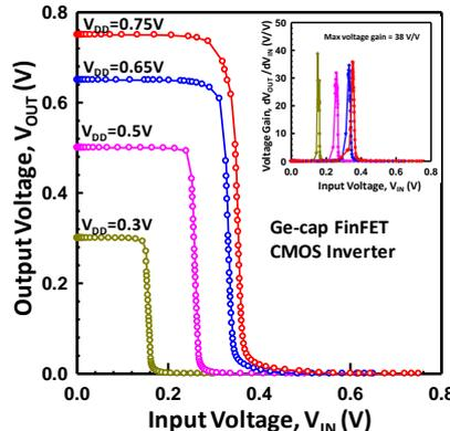
Fig. 6 Voltage transfer characteristics (VTC) of Ge-cap QW FinFET CMOS inverter with highest gain 38V/V
