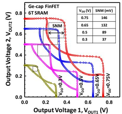
Fig. 7 Butterfly curves and static noise margin (SNM) values of Ge-cap QW FinFET 6T SRAM cells during read access
