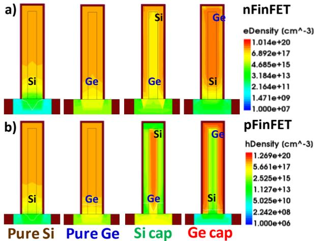
Fig. 3 a) Electron density of nFinFET and b) hole density of pFinFET for pure Si, pure Ge, Si-cap, and Ge-cap devices respectively under on-state condition ( $|V_D|=|V_G|=0.65\text{V}$ ).
