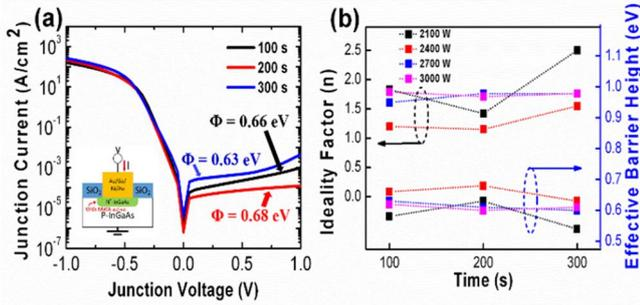
$\text{In}_{0.53}\text{Ga}_{0.47}\text{As}$  diodes with at MWA power of 2400 W for different annealing durations. The inset in (a) shows the schematic illustration of the junction cross section. (b) Ideality factor and effective barrier height with a variety of MWA conditions.
