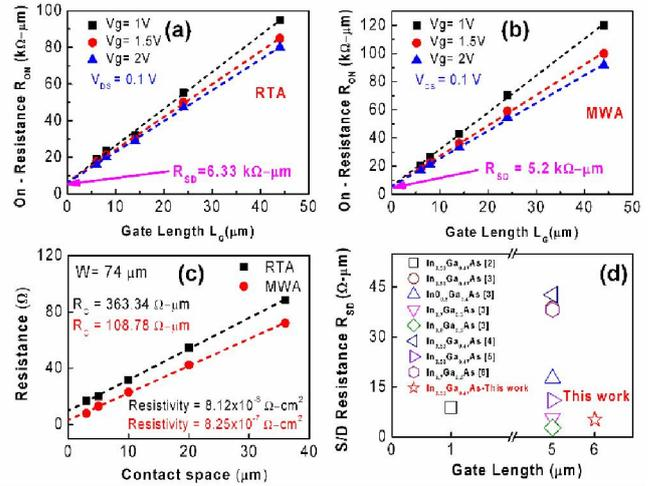
Fig. 4 Total resistance as a function of gate length for (a) RTA and (b) MWA samples. (c) TLM resistance versus spacing gap for RTA and MWA samples. (d) Benchmark S/D resistance of this work with reported values [2-6] on the InGaAs MOSFETs.
