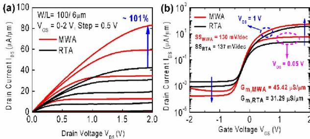
Fig. 3 (a) Output and (b) transfer characteristics of InGaAs MOSFETs fabricated with MWA and RTA processes.
