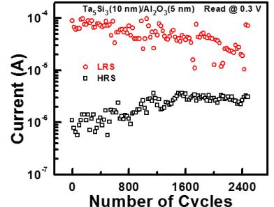
Fig.7 (b) Endurance test for DL device with Al<sub>2</sub>O<sub>3</sub> 5nm thickness measured at room temperature.
