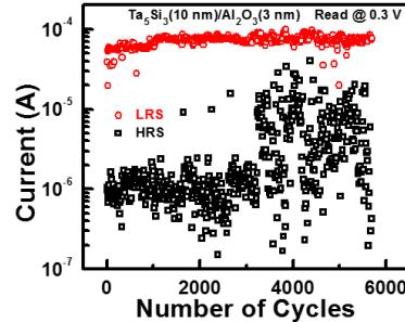
Fig.7 (a) Endurance test for DL device with Al<sub>2</sub>O<sub>3</sub> 3 nm thickness measured at room temperature.
