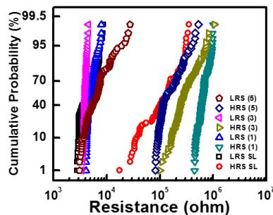
Fig.5 Distribution of resistances in HRS and LRS for 1000 sweep cycles for SL and DL devices.
