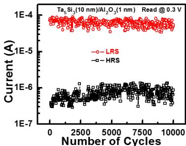
Fig.6 (b) Endurance test for DL devices measured at room temperature.
