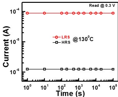
Fig.8 Retention behavior measured at temperature of 130°C for DL device.
