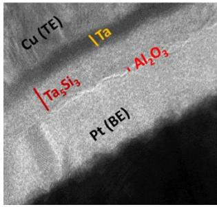
Fig.1 Cross-sectional TEM image of Cu/Ta<sub>5</sub>Si<sub>3</sub>/Al<sub>2</sub>O<sub>3</sub>/Pt device.
