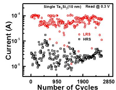
Fig.6 (a) Endurance test for SL devices measured at room temperature.
