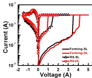
Fig.2 Forming process and I-V switching curves of the SL and DL devices.
