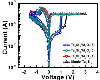
Fig.4 I-V switching curves of single Ta<sub>5</sub>Si<sub>3</sub> device and with Al<sub>2</sub>O<sub>3</sub> thickness (from 1nm to 5 nm)
