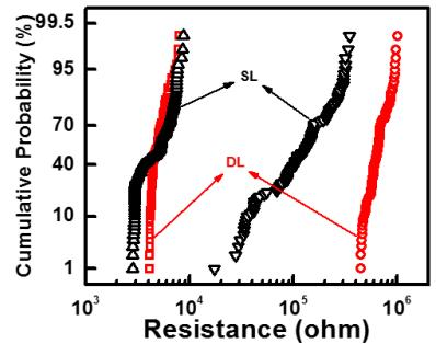
Fig.3 Distribution of resistances in HRS and LRS for 1000 sweep cycles.
