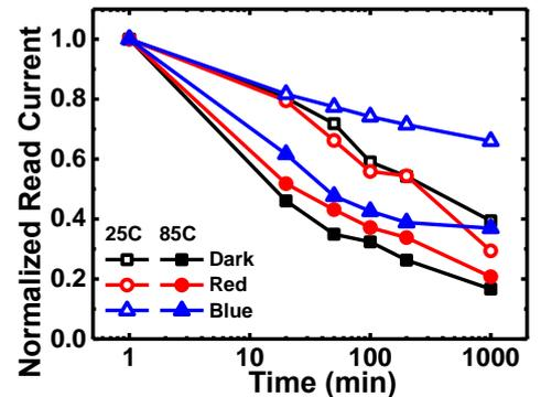
Fig. 10 Electron discharging on cells programmed under different triggering lights. Short wavelength light seems to promote trapping to deeper states for cells in the programmed states, leading to less charge lost.
