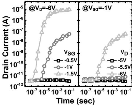
Fig. 4 Time to program. Characteristics under different  $V_{SG}$ ,  $V_D$ . Program can be complete within  $100\mu\text{sec}$
