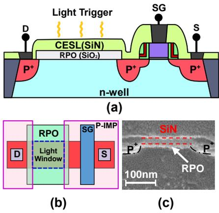
Fig. 1 (a) Illustration of the cross-section of gateless-anti-fuse memory cell. (b) layout of the memory cell. (c) The SEM picture of the gateless storage node.
