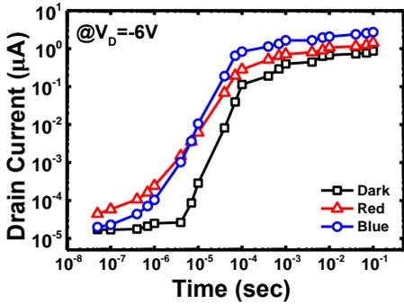
Fig. 6 Time to program under different triggering light suggested that initial leakage current can affect programming speed of this gate-less transistor.
