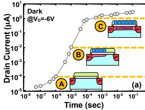
Fig.5 (a) Different states of programming levels. (b) Read current vs  $V_D$  at different stages of p-channel gate-less transistor. As the channel extends from left to right gradually at different programming states, its  $V_D$  dependence changes, as expected.
