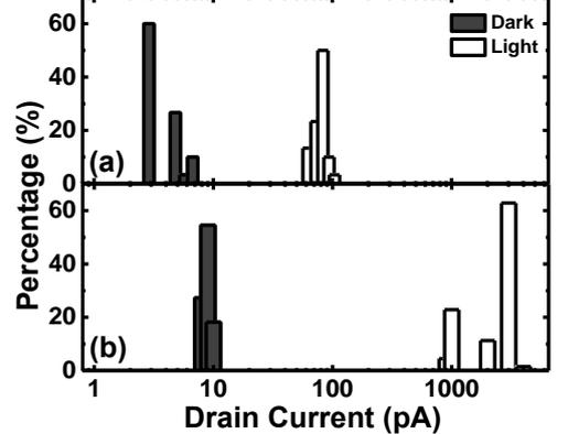
Fig. 8 Read current distribution after (a) 1 programming pulse of  $0.1\mu\text{sec}$  and (b) that after 10 pulses, resulting in large difference.
