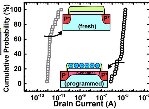
Fig. 2 Read current distribution of a fresh cell, without electrons in SiN layer, and that of cells in their programmed state, with electrons trapped in the SiN layer.
