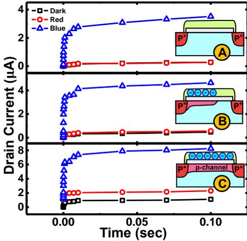
Fig. 7 Time to program characteristics from A, B, C states under triggering lights of different wavelength.
