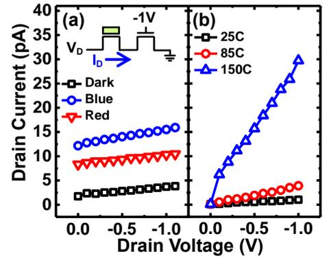
Fig. 3 Initial read current characteristics (a) that measured at dark and under the excitation of triggering lights and (b) that at different temperature.
