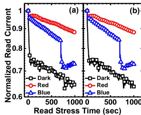
Fig. 9 Read disturbance tests performed (a) at dark and (b) under different type of light source. Data suggest triggering light enhance read stress immunity.
