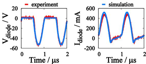
(a) Rectification waveforms at 1 MHz sinusoidal input.
