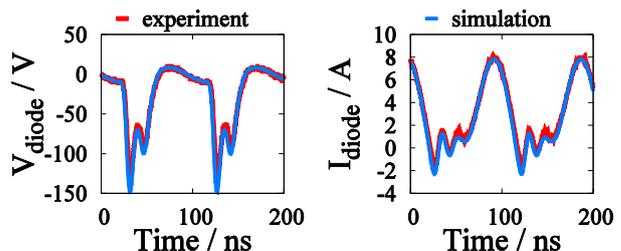
Fig. 5 Measurement and simulated waveforms about half-wave rectification at 10 MHz, 200 V<sub>pp</sub> input and 10 A max current. Simulating with parasitic inductances.
