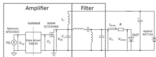
Fig. 2 Proposed measurement circuit using SiC MOSFET and LC resonant filter.
