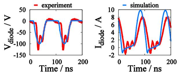
Fig. 4 Measurement and simulated waveforms about half-wave rectification at 10 MHz, 200 V<sub>pp</sub> input and 10 A max current.
