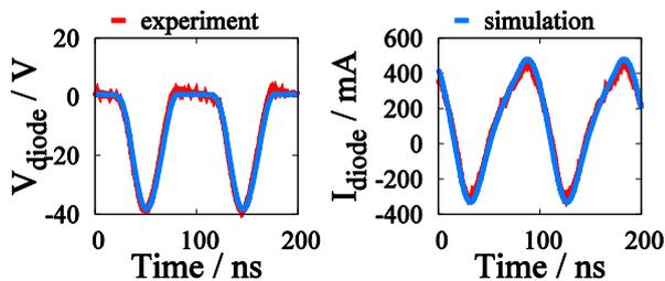
(b) Rectification waveforms at 10 MHz sinusoidal wave input.
