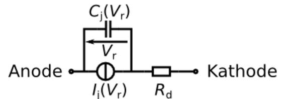
Fig. 1 Equivalent circuit of device modeling for SiC SBD.
