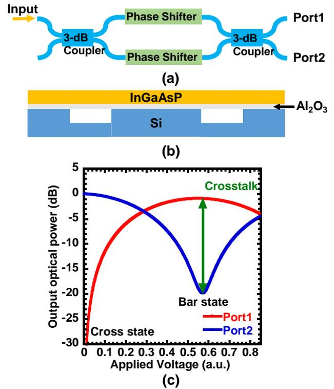
Fig. 1 (a) Schematic of MZI optical switch, (b) cross-section of InGaAsP/Si hybrid MOS optical phase shifter, and (c) crosstalk at bar state of MZI optical switch.
