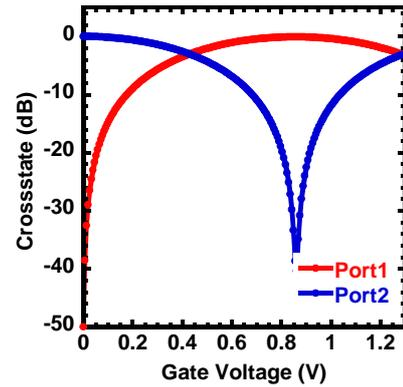
Fig. 3 The switching characteristics of MZI optical switch based on the InGaAsP/Si hybrid MOS optical phase shifter.
