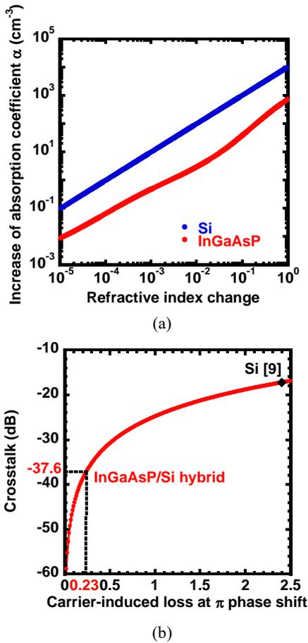
Fig. 2 (a) The relationship between the changes in refractive index and absorption coefficient and (b) the relationship between the carrier-induced absorption loss at  $\pi$  phase shift and the crosstalk of the optical switch.
