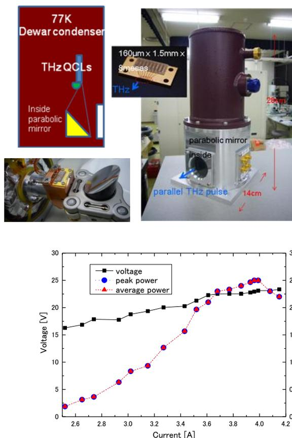
Fig. 1 Photographs of Dewar condenser with typical L-I-V curves.
