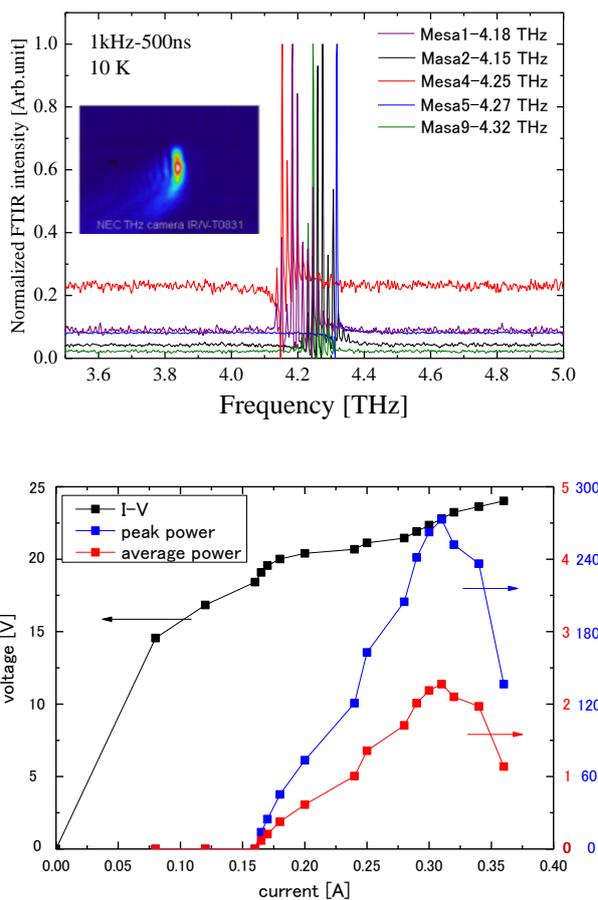
Fig. 2 Laing spectrum, THz camera image, and one typical L-I-V curves of our recently large output THz QCLs at 10 K operation.
