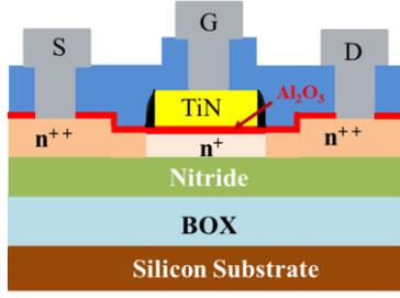
**Fig.1** Schematic of n-type channel Junctionless FET (JLFET) transistor with raised source/drain and gate spacer.
