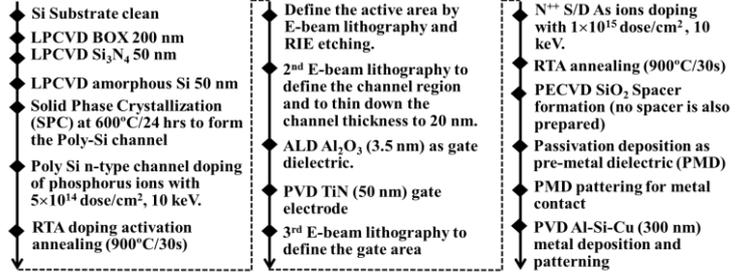
**Fig.2** Fabrication process and deposition conditions for the n-type JLFETs with raised source/drain and gate spacer. Without raised S/D or without gate spacer JLFETs are also prepared for the comparison.
