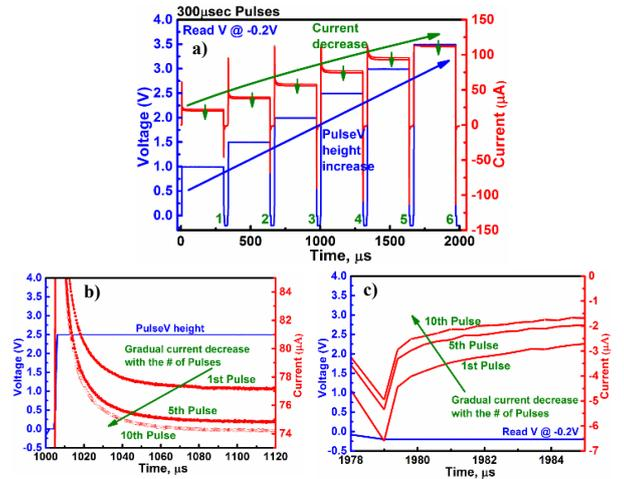
Fig. 6 Pulse measurements of 5μm-size Pt/SiO<sub>x</sub>/ZnO/Pt devices in RESET regime; Current read at -0.2V.
