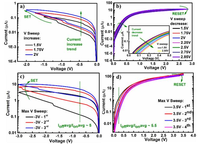
Fig. 4 Multilevel resistive switching I-V characteristics of 5μm-size Pt/SiO<sub>x</sub>/ZnO/Pt devices
