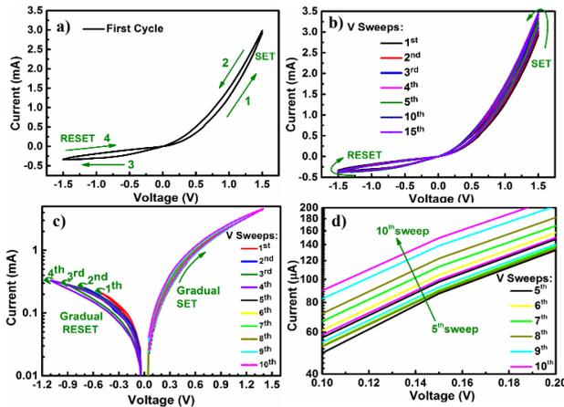
Fig. 2 Multilevel resistive switching I-V characteristics of 100μm-size Pt/SiO<sub>x</sub>/ZnO/Pt devices
