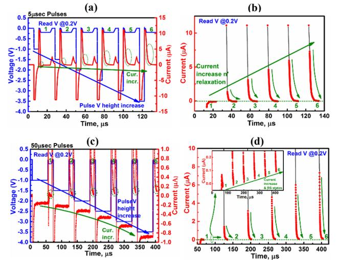
Fig. 5 Pulse measurements of 5μm-size Pt/SiO<sub>x</sub>/ZnO/Pt devices in SET regime; Current read at -0.2V.
