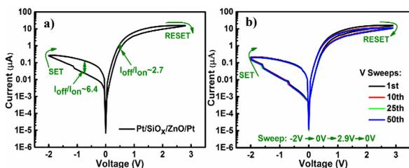
Fig. 3 Resistive switching hysteresis loops I-V characteristics of 5μm-size Pt/SiO<sub>x</sub>/ZnO/Pt devices
