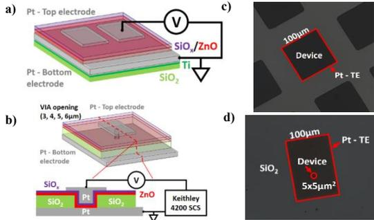
Fig. 1 Schemes of the Pt/SiO<sub>x</sub>/ZnO/Pt devices and its optical microscope view
