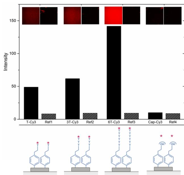
Fig. 2 Fluorescence intensity of functionalized gold electrodes after DNA synthesis in a commercial DNA synthesizer. Three different poly-T lengths with a terminal Cy3 group were synthesized on samples 1, 2 and 3. Sample 4 was first capped, after which a synthesis run with Cy3 phosphoramidite was performed. The negative reference electrode in each synthesis run was a non-functionalized electrode. The fluorescence microscopy images are shown in inset.
