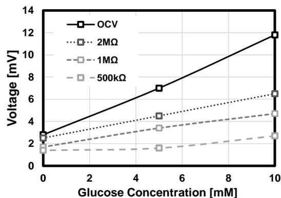
Fig. 5. Output voltage as a function of glucose concentrations.
