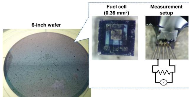
Fig. 3. Photograph of the developed prototype and measurement setup.
