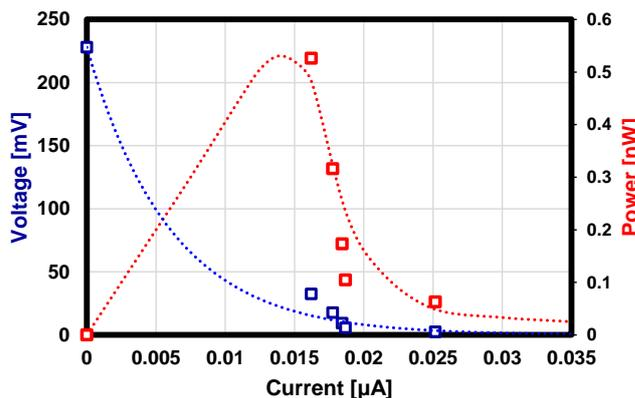
Fig. 4. Output voltage and power dependence on output current.
