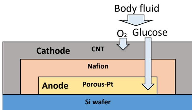
Fig. 1. Conceptual image of the developed fuel cell.
