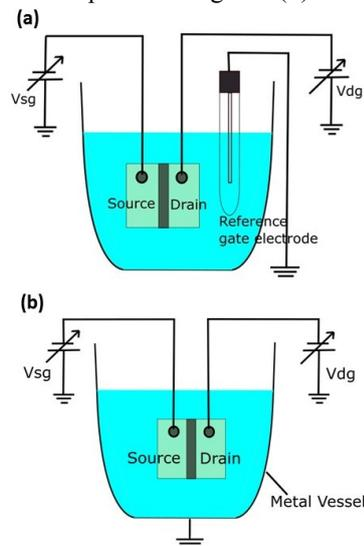
Figure 1: Common Gate configuration using (a) Ag/AgCl reference gate electrode and (b) Metal vessel gate
