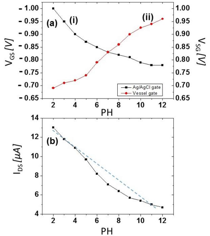
Figure 3: pH sensitivity of (a(i)) Ag/AgCl gate (a(ii)) Common-gate in metal vessel and (c) Current sensitivity across pH measured in metal vessel
