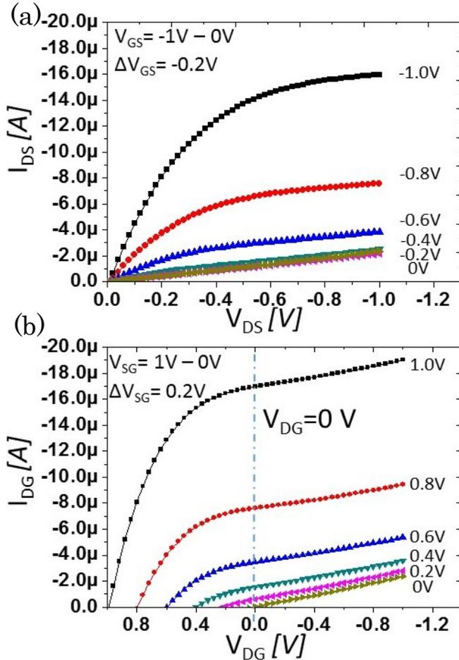
Figure 2: I-V Characteristics of (a) Common-source and (b) Common-Gate configuration measured in vessel
