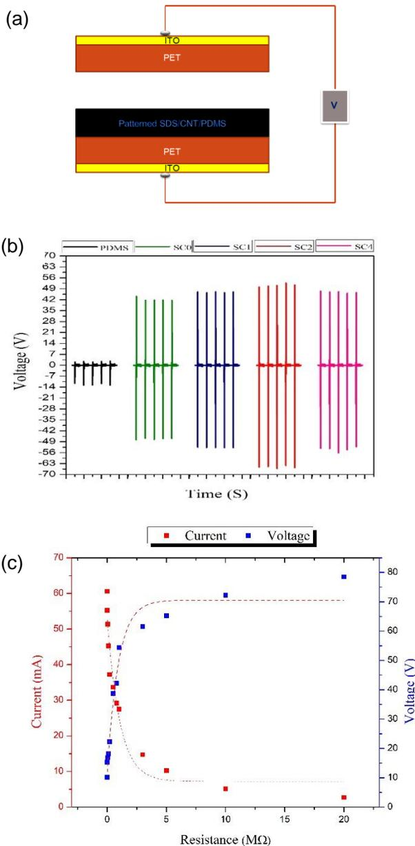
Fig. 1 (a) Schematic view of the TENG, (b) open-circuit voltage output of the TENG devices and (c) output voltage and current of the TENG (SC2) device under different external loads
