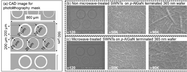
Fig. 3 (a) Fabricated CTLM structure to measure ohmic contact properties on p-AlGaIn using Chrome (Cr) photomask designed using computer-aided design program. (b) Pristine SWNT and (c) MWT-SWNT films with arrays of CTLM patterns on p-AlGaIn epi wafers.
