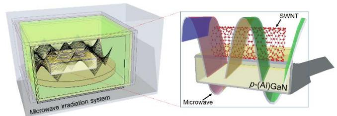
Fig. 1 Schematic illustrations of the MWT applied to SWNT TCEs for ohmic contact to the p-AlGaN. The magnified image on the right-hand side shows that microwave can be irradiated to SWNTs on the p-AlGaN using the microwave irradiation system.
