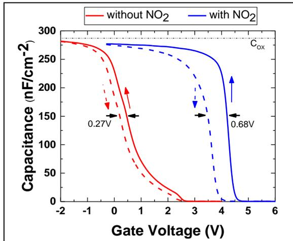
Fig. 2 C-V characteristics of MOS diodes without NO<sub>2</sub> hole doping (red) and with NO<sub>2</sub> hole doping (blue). Measurement frequency is 1 kHz.
