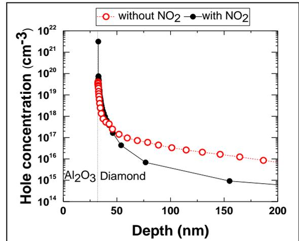
Fig. 3 Depth profile of the hole concentrations of the MOS diodes with and without NO<sub>2</sub> hole doping obtained from C-V measurements.
