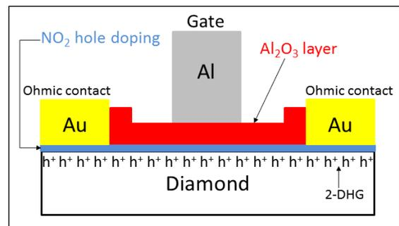
Fig.1 Schematic cross section of NO<sub>2</sub> doped diamond MOS diode. NO<sub>2</sub> hole doping is made on hydrogen terminated diamond. Al<sub>2</sub>O<sub>3</sub> layer is used as an insulating layer of MOS diode.
