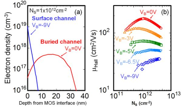
Fig. 4 (a) simulated carrier distribution of the SiC MOSFETs at the MOS interface with applying body bias (b)  $\mu_{\text{Hall}}$  in channel region as a function of  $N_S$  with the body bias. The dose of N was  $8 \times 10^{12} \text{ cm}^{-2}$ .
