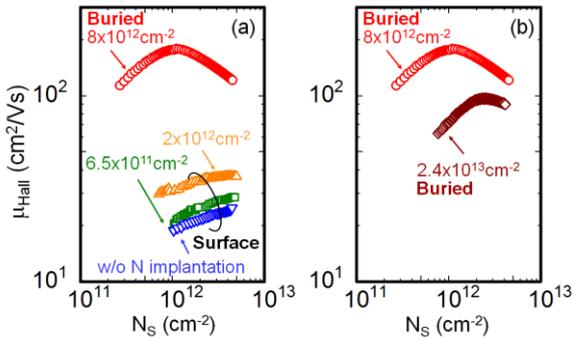
Fig. 3 (a)  $\mu_{\text{Hall}}$  in channel region as a function of  $N_S$  for the surface channel and buried channel devices. The device whose dose of N is  $8 \times 10^{12} \text{ cm}^{-2}$  works as the a buried channel device. (b)  $\mu_{\text{Hall}}$  in channel region as a function of  $N_S$  for the buried channel devices. The dose of N is  $8 \times 10^{12} \text{ cm}^{-2}$  and  $2.4 \times 10^{13} \text{ cm}^{-2}$ , respectively.
