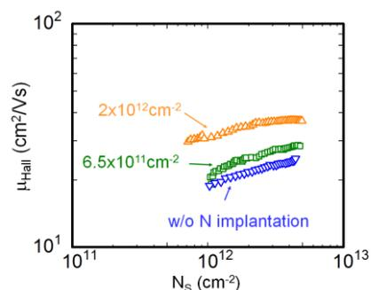
Fig. 2  $\mu_{\text{Hall}}$  in channel region as a function of  $N_s$  for the devices with the dose of N from 0 to  $2 \times 10^{12} \text{ cm}^{-2}$
