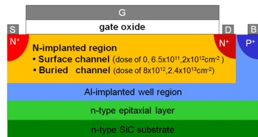
Fig. 1 Schematic of the fabricated SiC MOSFETs with N-implanted region on Al-implanted well region.
