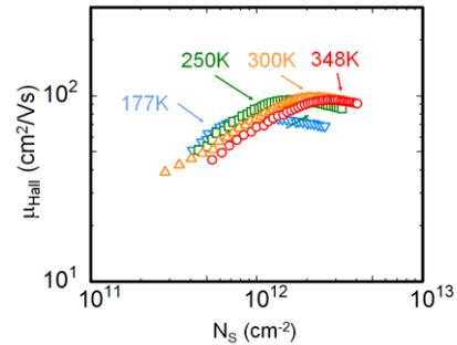
Fig. 5  $\mu_{\text{Hall}}$  in channel region as a function of  $N_S$  with changing temperature. The dose of N was  $2.4 \times 10^{13} \text{ cm}^{-2}$ .
