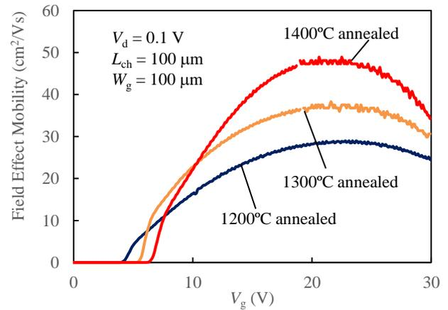
Fig. 4 Field effect mobility curves of fabricated GaN MOSFETs with different Mg activation annealing temperature.
