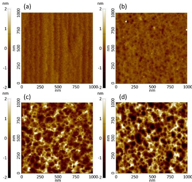
Fig. 2 AFM images of GaN surface. (a)  $[Mg] = 1 \times 10^{18}$  cm<sup>-3</sup> as implanted wafer, (b) after 1200°C annealing, (c) after 1300°C annealing, and (d) after 1400°C annealing.
