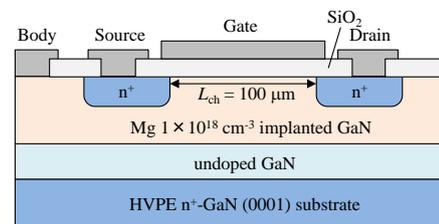
Fig. 1 Schematic cross section of lateral GaN MOSFETs with all-implantation process. The long channel design was used to extract MOS channel characteristics.
