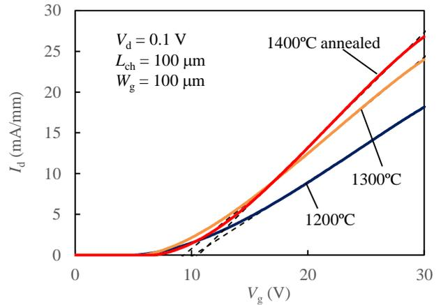
Fig. 3  $I_d$ - $V_g$  transfer characteristics of fabricated GaN MOSFETs with different Mg activation annealing temperature.
