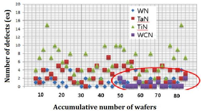
Fig. 3 Number of defects vs accumulative number of wafers corresponding to 4 different Cu TSVs with WN, TaN, TiN, and WCN diffusion barriers
