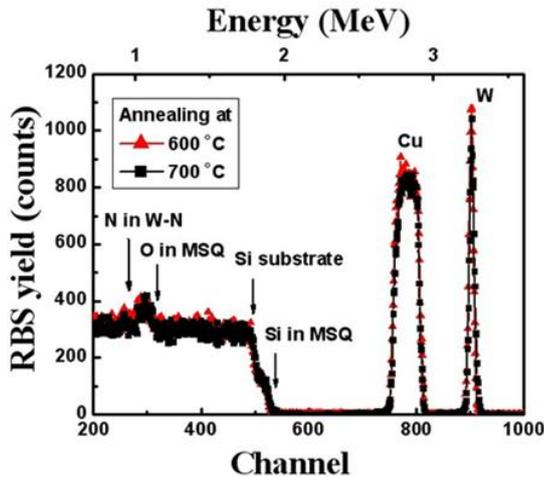
Fig. 2 Rutherford backscattering of Cu/WCN/MSQ/Si structure at the annealing temperatures, 600 and 700 for 30 min
