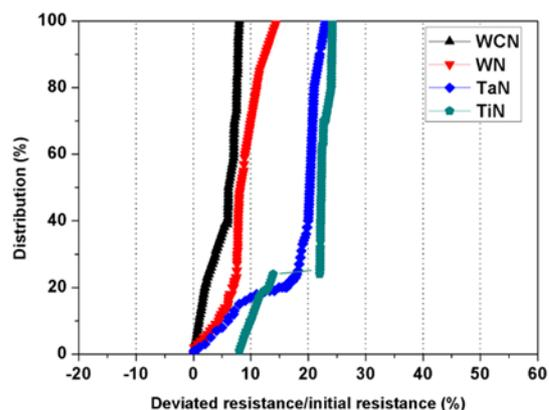
Fig. 1 Distribution of contact resistance vs percent of deviated resistance/initial resistance
