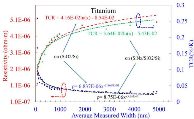
Fig. 2 Temperature coefficient of resistance (TCR) and resistivity ( $\rho$ ) with the variation of average measured width for Ti thermistor with two different substrates.
