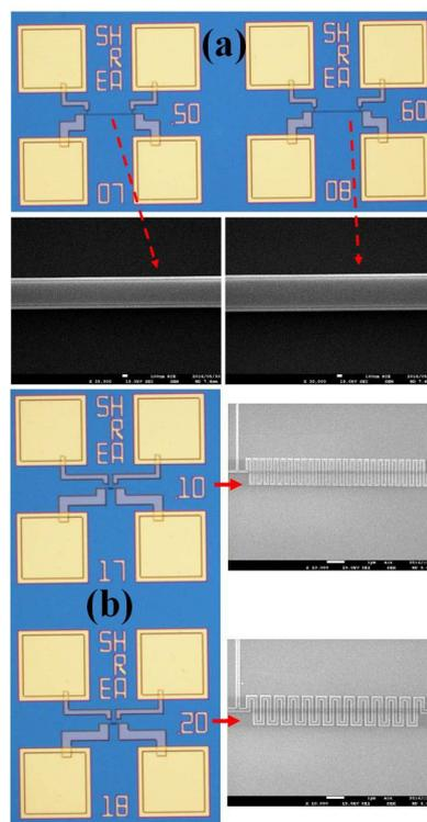
Fig. 1 OM image with enlarged FESEM image of (a) straight and (b) meander Ti devices with Au pads fabricated for measurement of the width effect on the thermistor.
