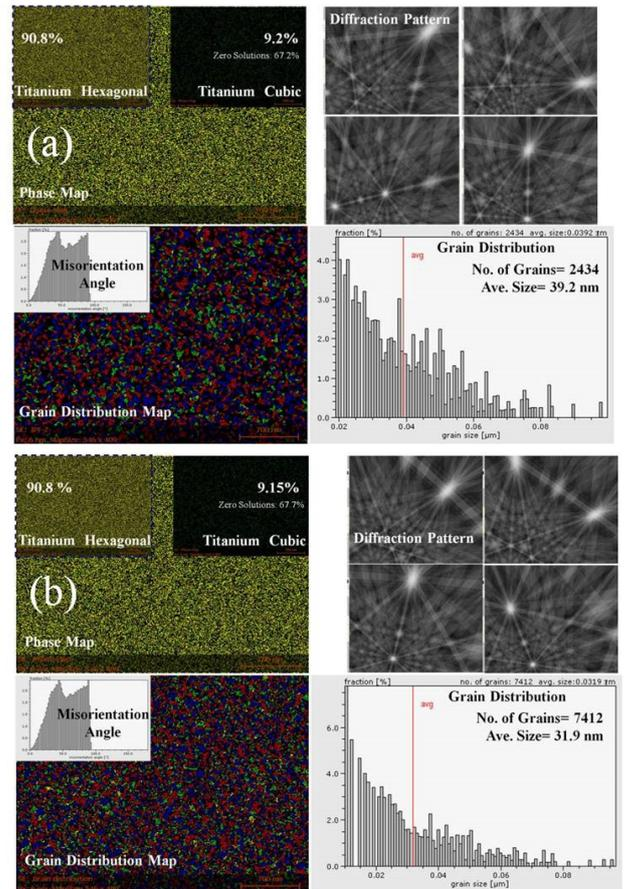
Fig. 3 Electron backscatter diffraction (EBSD) showing phase map, local diffraction patterns, grain distribution and average grain size for Ti (a) film ( $150 \times 150\ \mu\text{m}$  area) and (b) nanowire with width 100 nm.
